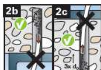
2b 2c Cleaning of the drill hole may be omitted when drilling vertically upwards or downwards. However, increase the drill hole depth by 30mm.
