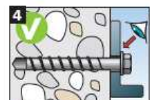
4 After screwing on, it must not be possible to turn the screw slightly. The screw head must rest on the attachment part and must not be damaged.
