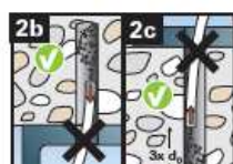
2b 2c Cleaning of the drill hole may be omitted when drilling vertically upwards or downwards. However, increase the drill hole depth by 30mm in this case.
