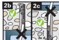
2b 2c Cleaning of the drill hole may be omitted when drilling vertically upwards or downwards. However, increase the drill hole depth by 30mm in this case.
