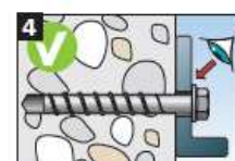
4 Once tightened, it must not be possible to turn the screw. The screw head must rest on the fixture and must not be damaged.
