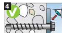
4 Once tightened, it must not be possible to turn the screw. The screw head must rest on the fixture and must not be damaged.
