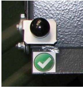
Backstop free (normal position)
