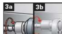
3a 3b Tighten the concrete screw with a socket spanner (spanner size 15). Observe the maximum tightening torques.
