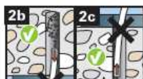
2b 2c Cleaning of the drill hole may be omitted when drilling vertically upwards or downwards. However, increase the drill hole depth by 30mm in this case.
